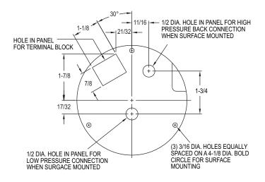
MOUNTING: The Series 605 Transmitter may be either panel mounted or surface mounted.
