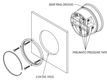
A. PANEL MOUNTING: Cut a 4-3/4<sup>~</sup> or 120 mm dia. hole in panel and insert the complete unit from the front. Slip on the mounting ring and install the split snap ring in the groove on the bezel. Seat the mounting ring against the snap ring and thread the four screws through the tapped holes. Tighten screws against rear of panel.
