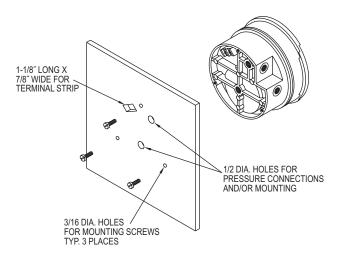
B. SURFACE MOUNTING: Drill (3) 3/16" dia. holes for mounting screws and cut (1) 7/8" x 1-1/8" hole for access to terminal strip as shown in hole location drawing. Insert screws from rear of panel and thread into tapped holes on back of transmitter case. If rear pressure connections are to be used, make 1/2" dia. holes located as shown in hole location drawing in left column.
