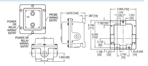
The MODEL LTC2 Tilt Switch Control Units offers a complete level control solution when used with a tilt switch probe such as the Series LTS. It offers a DPDT switch output as well as indicator lights to provide visual and output control of the level probe status
