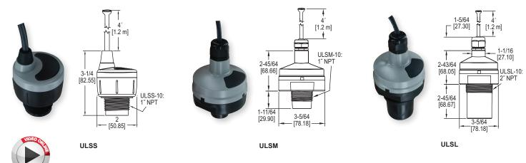
The Series ULSS Ultrasonic Level Sensor provides non-contact, continuous ultrasonic level measurement of fluids for short range applications. It has a 4.1' (1.2 m) measuring range with a 0.125" (3 mm) accuracy.
