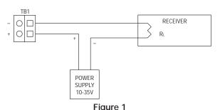
An external power supply delivering 10 to 35 VDC with a minimum current capability of 40 milliamps must be used to power the control loop in which the Magnesense transmitter is connected. Refer to Fig. 1 for connection of the power supply, transmitter and receiver. The range of appropriate receiver load resistances (RL) for the power supply voltage available is given by the formula and
