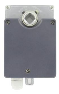
**DDA Series Direct Coupled Actuators** are non-spring return actuators that are perfect for positioning of dampers and valves in HVAC systems. Actuators are designed to accept floating control signals and come in a variety of power supplies. Actuators produce 17 to 70 in-lb (2 to 8 Nm) of torque. Contact factory for optional internal auxiliary switch.
